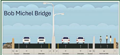
bridge, by combining two existing pedestrian/bike lanes into one, and by narrowing the traffic lanes by one foot each.
